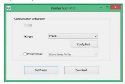
Connect the printer after "Config Port" via serial port, Ethernet port or parallel port, then proceed to "set printer" or "download".
