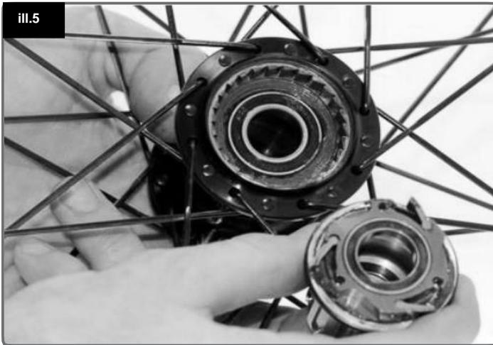
All components can now be inspected and replaced if necessary.
