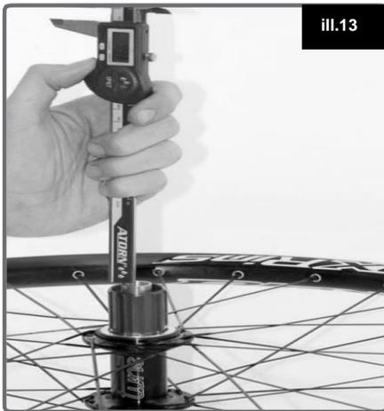
Subtract from the measured value (e.g. 9.8 mm) the insertion depth of the end cap (e.g. 9.2 mm). You will then receive the current game (here  $9.8 \text{ mm} - 9.2 \text{ mm} = 0.6 \text{ mm}$ ).
