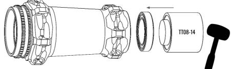
**Tech tips :** When you press your bearing, always make sure it's correctly aligned. If not, restart the process, and hammer more gently until the bearing is perfectly aligned.
