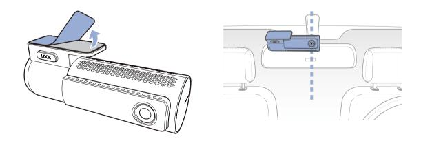
Adjust the angle of the lens by rotating the body of the front camera. We recommend pointing the lens slightly downwards (≈10° below horizontal), so as to record video with a 6:4 road to background ratio.
