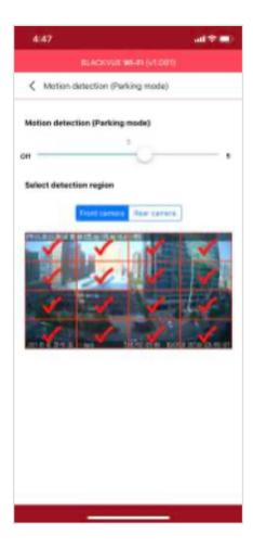
In Motion Detection Parking Mode the dashcam continuously buffers video and saves a parking recording when motion is detected in the dashcam's field of view.
