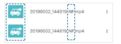
Recording file names include the date, time, recording type and camera direction.
