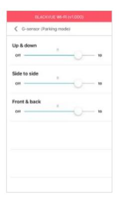
The G-sensor measures the movement of your vehicle through 3 axes – up and down, side to side, and front and back. When the G-sensor detects significant or sudden movement (such as an impact or collision) it will trigger an event recording. You can adjust the sensitivity so minor incidents and bumps don't trigger an event recording. To turn off event recordings by impact detection set the G-sensor sensitivity to off.
