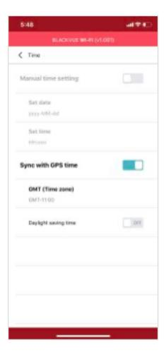
Select your time zone to auto-sync with GPS time or you can set the time and date manually after enabling **Manual time setting**.
