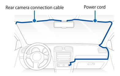
Turn on the engine. The BlackVue dashcam will power up and start recording. Video files are stored on the microSD card. When the microSD card fills up, the newest video files will start to replace the oldest video files (called loop recording) – so you will always have the most recent video files.
