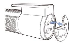
To insert the SIM card, remove the bracket from front camera. Then open SIM slot by using SIM eject tool.
