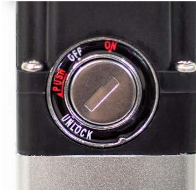
3. When your battery is in the UNLOCKED position, you will be able to remove it from the frame and the power will not be active. **Use caution when unlocking and removing your battery from the frame, as it may slide out when the bike is folded. If your battery impacts the ground and is damaged, discontinue use and contact Lectric eBikes immediately.**
