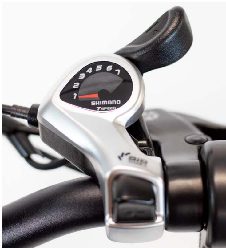
**Do not change gears too quickly as doing so could cause the chain to fall off and the rider to lose control, which could result in serious injury. If the chain falls off, turn the bike off before fixing the chain. If you do not and the motor turns on you could sustain serious injury.**
