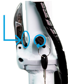
Locking Pin protruding through frame
