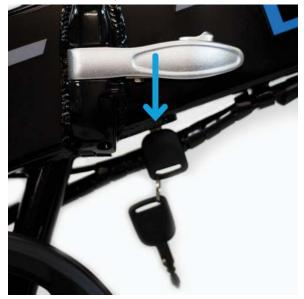
8. Push the key in firmly and turn the key clockwise to lock the battery to the bike and turn it to the ON position. You will not be able to remove the keys from the battery in this position.
