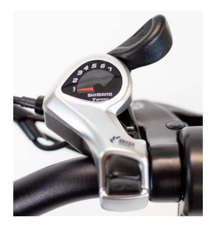
Do not change gears too quickly as doing so could cause the chain to fall off and the rider to lose control, which could result in serious injury. If the chain falls off, turn the bike off before fixing the chain. If you do not and the motor turns on you could sustain serious injury.
