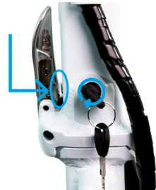
Locking Pin protruding through frame
