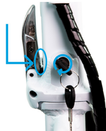
Locking Pin protruding through frame
