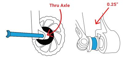
6. Align the quick release lever with the cutout in the thru axle endcap. Begin turning the lever clockwise, keeping the lever open and in the slot.
