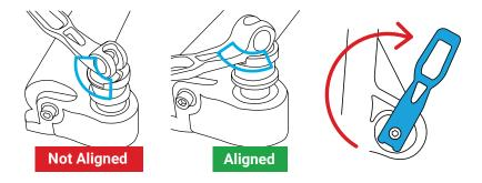
7. When you cannot screw the thru axle in any further, close the lever by folding it 180 degrees. There should be resistance building when the lever is closed, if there is no resistance repeat steps 5-7 again.
