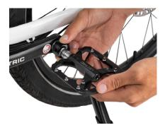
1. Pull the spring-loaded sleeve and insert the pedal axle while aligning the hex pattern.
