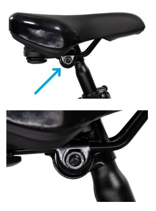
**Seat angle adjustment:** Most people prefer a horizontal seat; but you may prefer the seat nose angled slightly up or down. Loosen the clamp bolt to allow any serrations on the clamp mechanism to disengage before changing the seat angle, and to fully re-engage the serrations before you tighten the clamp bolt to the recommended "Tightening Torque" on page 25.
