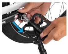
1. Pull the spring-loaded sleeve while also pulling the pedal out from the hex slot.
