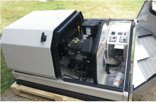
they switch ON and OFF automatically as needed. A 12,500 watt standby unit, for instance, costs about \$4500. These units can't be moved around, but they do offer the lowest cost-per-watt figures of all generators, along with quiet operation, automatic switching and a quality of power output that's worth taking a closer look at. More on this later.
