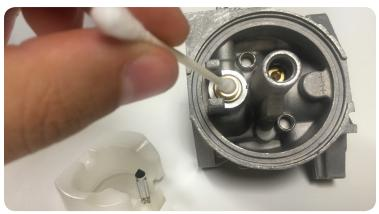
A cloth with some WD-40 can be used to clean the rubber tip of the float needle also. Be sure to wash both the needle and needle seat areas with aerosol spray cleaner to eliminate any remaining debris after cleaning. Re-assembly should solve your flooding problem.
