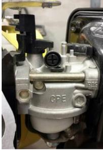
2. Using a small flat head screwdriver, pop the plastic pilot jet out from the carburetor body. On 270cc + engines there may be a spacer between the black plastic screw and pilot jet.
