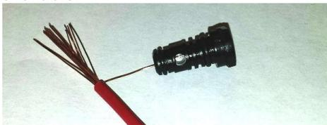
4. Reinstall pilot jet making sure the groove on top of the jet is inline with the airflow.
