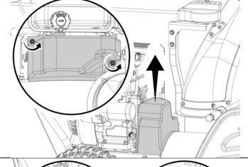
2. Remove the 2 bolts (20 mm/30 mm) holding the belt guard. If your snow blower currently has a single sided belt guard please replace it with a double sided belt guard as part of this repair.
