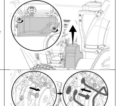
3. Once installed, make sure there is equal distance on both sides between the pulley and the guard. (1/16 to 3/16" or 2-5mm). If the distance needs to be adjusted, carefully use a long socket extension or pry bar to adjust the guard. Be careful not to damage the belt or pully.
