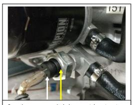
Corrosion prone areas include sensor tab root vent (white) and plastic/metal seam (yellow)
