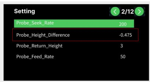
Move to Settings->Grbl Setting, and check if the Probe\_Height\_Difference value match the result of the Z probe calibration
