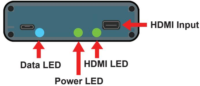
**Step 1:** Start the vehicle, the interface should have one blinking blue LED and two steady lit green LED lights.
