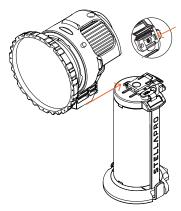
Push light onto battery until it snaps into place
